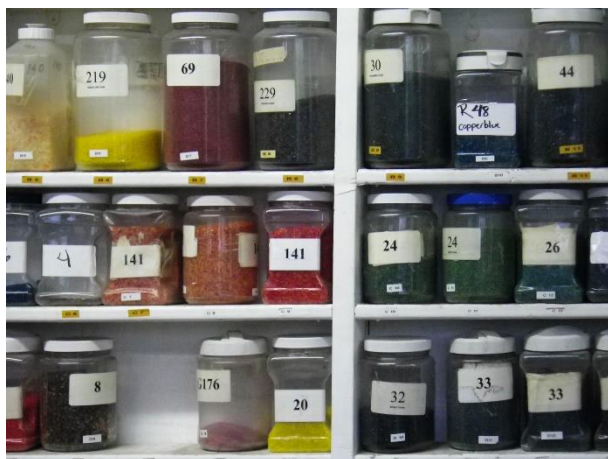
Metals and other chemicals added to silica to provide color
