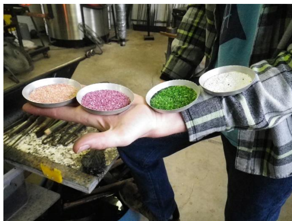
Metals and other chemicals added to silica to provide color
